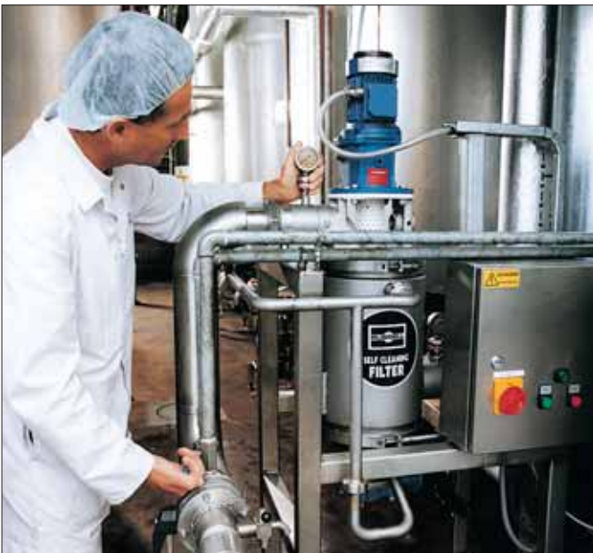
Self-Cleaning Russell Eco Filters® aid quality control procedures for filtering liquid chocolate at Walls Ice Cream.
