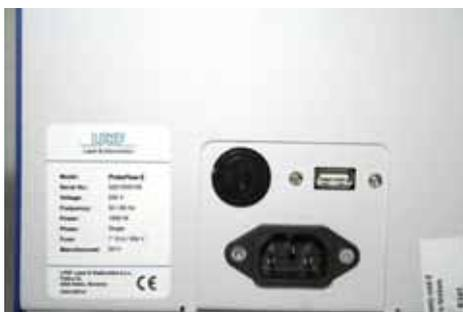
AUSBconnectionporttypeAisplacedontherearside of the oven.
