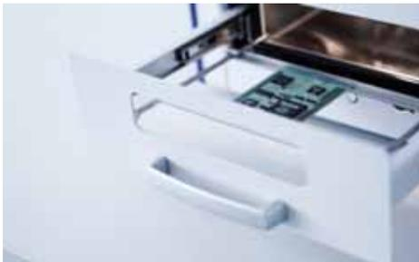
Mounting of PCB's up to the size of 160×200mm (6.3"×7.9") is possible. The two securing strips slide easily onto carriers. To prevent uncontrolled motion, the strips are fixed with pin screws.
