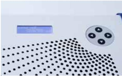
Menu selection from the four-line LCD using the keyboard is logical, i.e. the direction arrows move the selection on the LCD in the appropriate direction.
